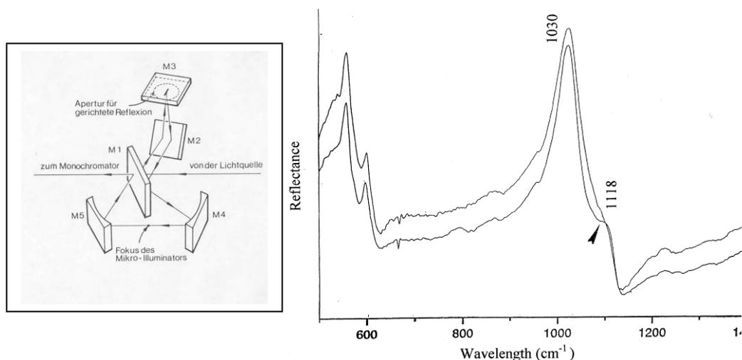
Fig. 18 and 19 - Construction scheme of a reflection equipment used in a FTIR spectrometer (left) and FTIR reflection spectra showing the characteristic differences (shoulder at 1180 cm<sup>-1</sup>) between Asian and African ivory (right).
