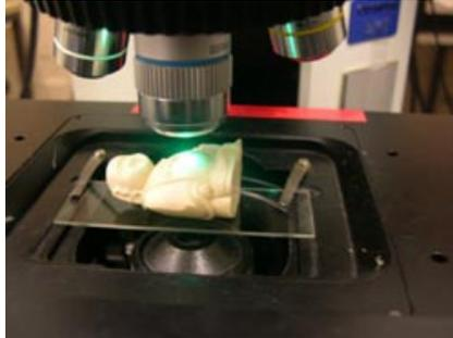
Fig. 2 - Non- destructive investigation of netsuke by Laser Raman Spectroscopy equipped with a confocal microscope
