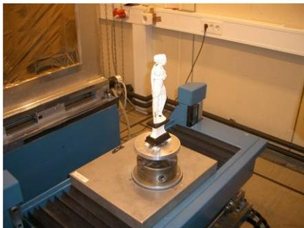
Fig. 9: Ivory object mounted on the sample stage of the XCT machine at BAM, Berlin
