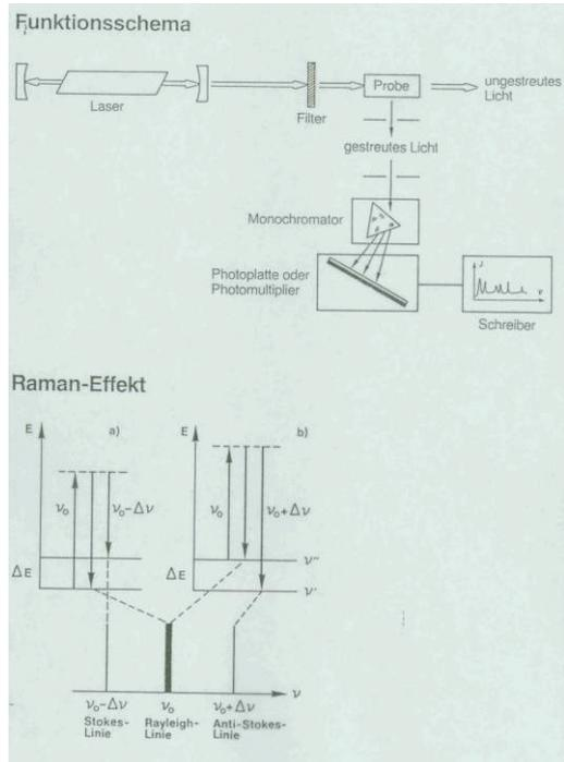
Fig. 20 - Schematic drawing of the working principle of Raman spectroscopy
