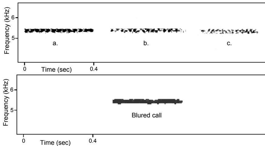
**Figure 4:** Improving detection of honeycomb-shaped calls with blur filtering and HMMs. In the top image, calls a, b, and c are each from the same species of cricket. Their uneven pixel cluster shapes result in poorer performance with the contour feature vector method. By first applying a blur filter, this unevenness becomes smoothed, and the calls become more readily classified with the contour feature vector method.
