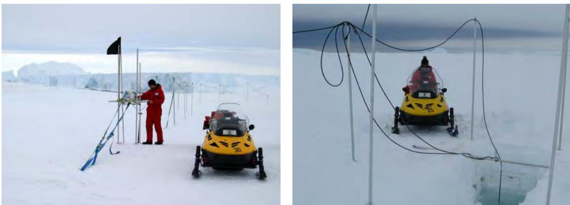
**Figure 7:** Single hydrophone deployment through sea ice.
