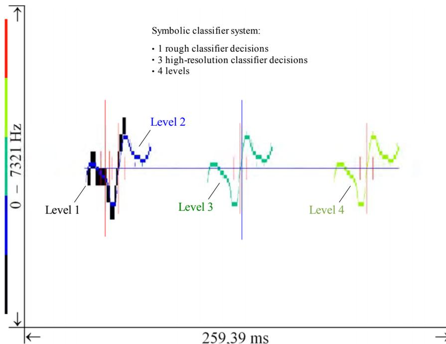
**Figure 10:** Symbolic hierarchical classifier system for a sequence of syllables. Hierarchical symbolic classifier systems can be quicker and more accurate than simple classifiers. They can be designed to recognize entire sequences of elements. Tolerance parameters enable fuzzy pattern recognition. The levels of the internal hierarchy are color coded.
