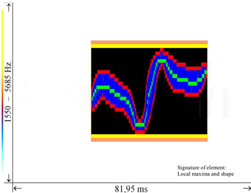
**Figure 7:** Template based signature in highlight mode. The signature was derived manually from one single example by applying a template to the spectrogram in figure 3. Green are local maxima of Fourier coefficients. Red is the shape of the acoustic event. Blue are above threshold coefficients important for pattern formation algorithms.
