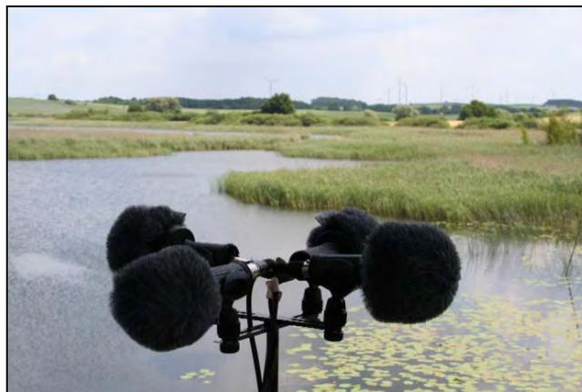
**Figure 2:** Microphone array for acoustic monitoring. Four cardioic microphones (Sennheiser ME 64 or Beyerdynamic MC 930) were placed in cross configuration.
