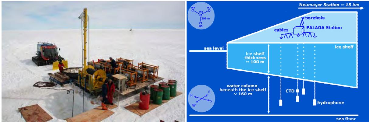
**Figure 5:** Hot Water drilling equipment and hydrophone array layout.
