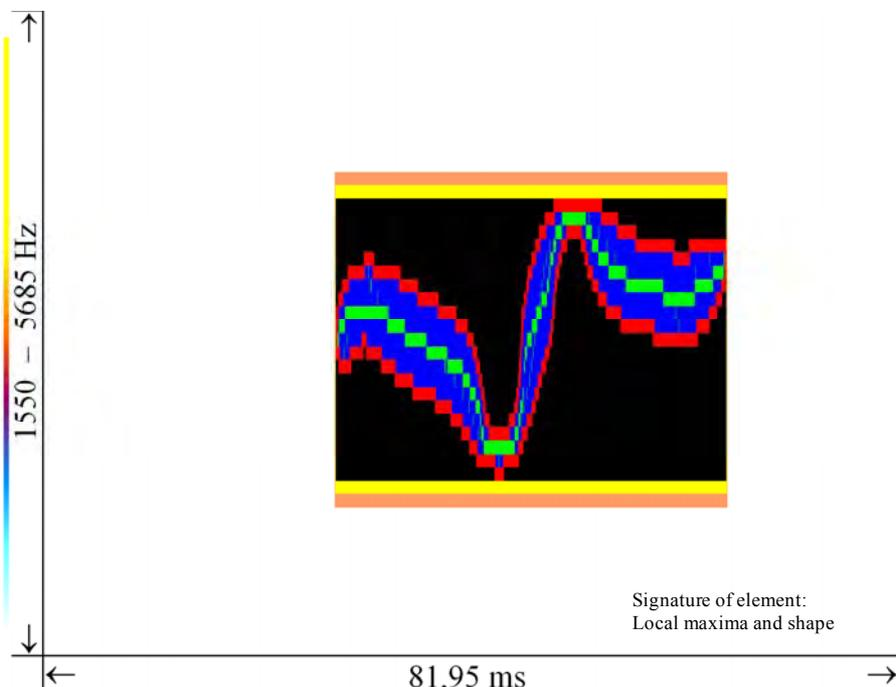
**Figure 8:** Induced signature in highlight mode. The signature was induced by merging twelve similar patterns found by a classifier using the signature in figure 4. Induced signatures usually perform better than template based signatures though they look similar at first sight.
