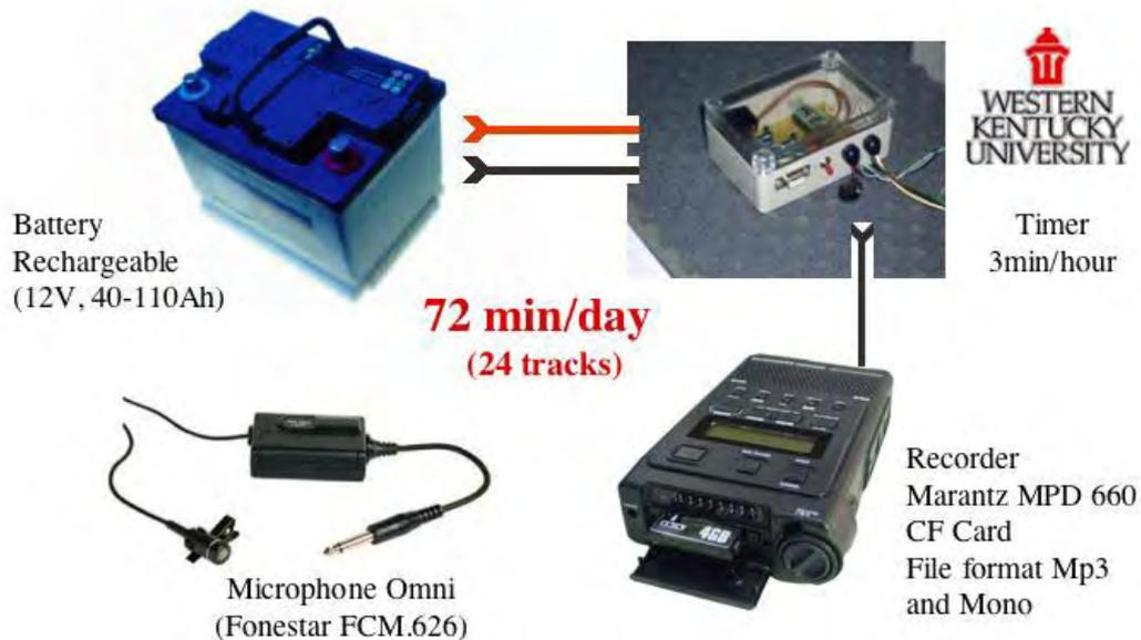
**Figure 3:** Diagram of the automated recording system.
