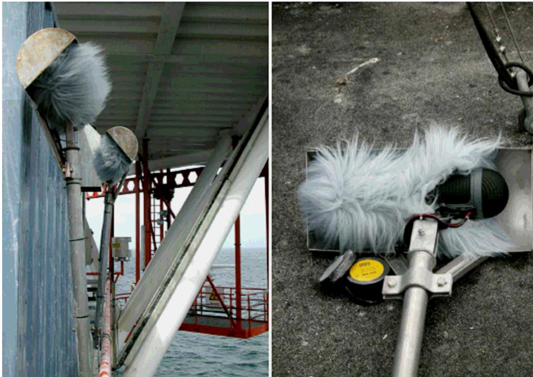
Figure 1: Bat detector and microphone with windshield and mic muff on FINO 1.
