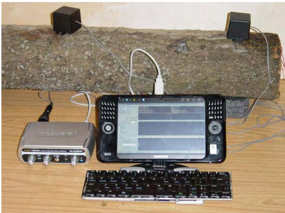
**Figure 7:** Latest implementation of IBIS using Samsung Q1 ultra-portable PC and external sound card.
