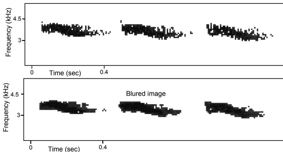
**Figure 5:** Improving detection of calls with uneven edges with blur filtering and HMMs. A sequence of calls is shown in the top image without applying the blur filter. Their rough edges creates difficulty for the contour feature vector. By smoothing the image with a blur filter, these edges become smoother and improve the performance of the contour feature vector.
