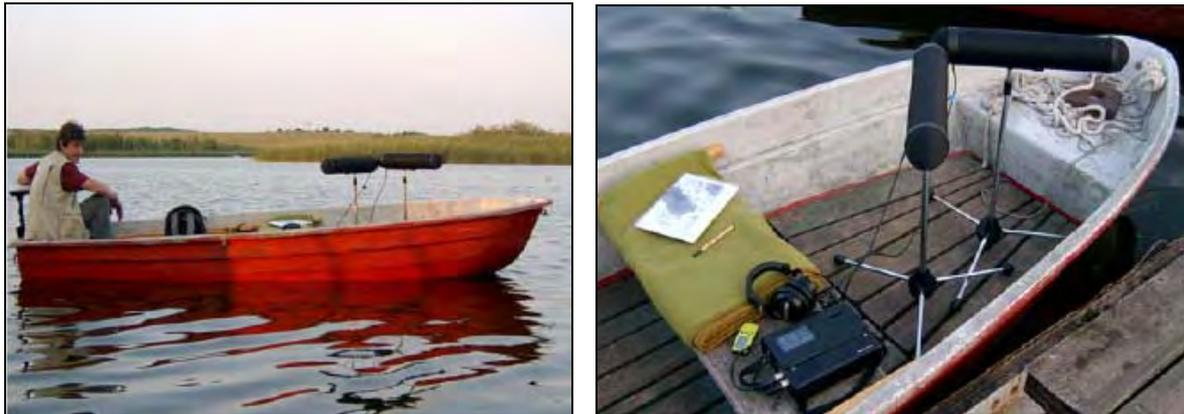
**Figure 8:** Equipment for GPS-supported acoustic monitoring of Savi's warblers. A small boat equipped with an electromotor was driven at low speed along the border of the reed belt. During the movement, continuous acoustic recordings were taken by two directional microphones arranged at a 90 degree angle. The position of the boat was determined simultaneously by GPS.
