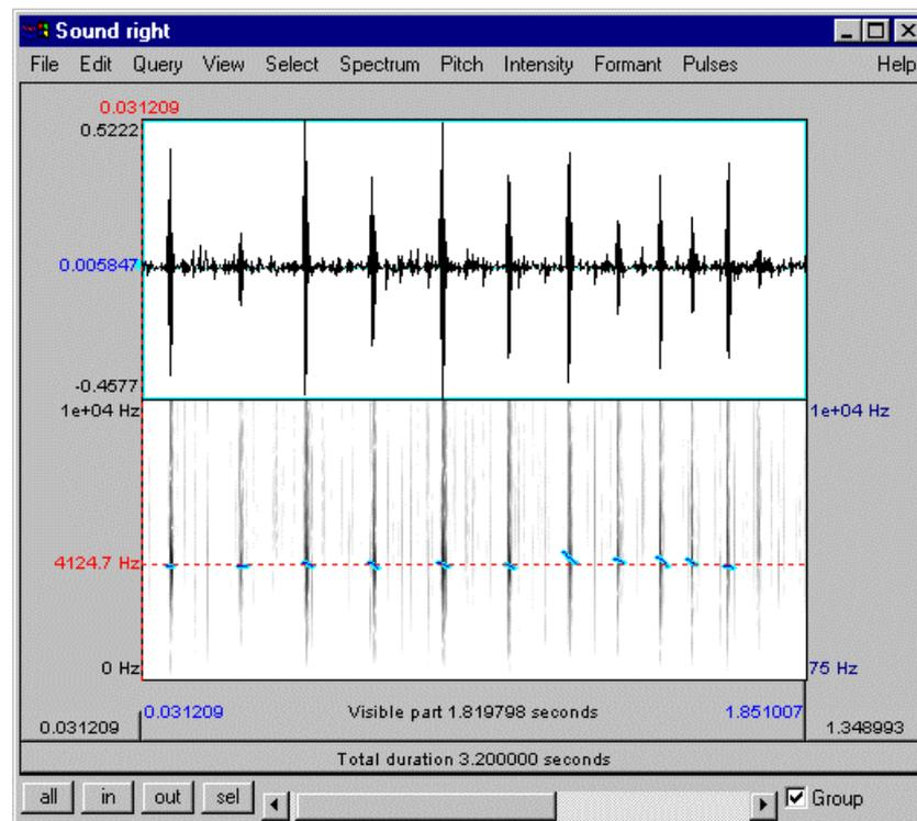
**Figure 3:** Only the right channel of the bat detector (divide-by-ten) is used for pitch analyses. The screenshot shows oscillogram (top, intensity vs. time) and spectrogram (bottom half) with pitch (blue). The dominating frequency of 4125 Hz x 10 ~ 41 kHz identifies this individual as a Nathusius's Pipistrelle - *Pipistrellus nathusii*.
