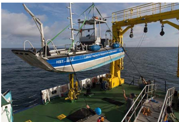
Figure 4: Deploying the working boat Klaashahn from EMB (© Kube/IOW).
