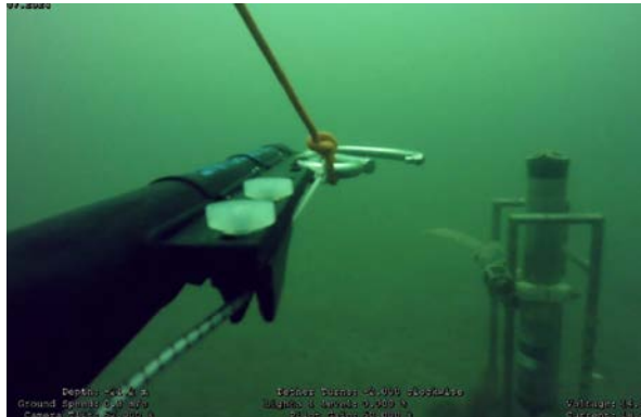
Figure 5: Dense point cloud of a photomosaic reconstruction showing an Fi103 rocket war head with 1000kg of explosives when intact. The shown object is open and almost half of the explosives are already dissolved into the water. New version of the ROV mooring recovery hook and a video screen shot showing the recovery of an acoustic current profiler. The hook is placed and pulled out of the deployment arm. ROV and hooked-in device are recovered separately afterwards.
