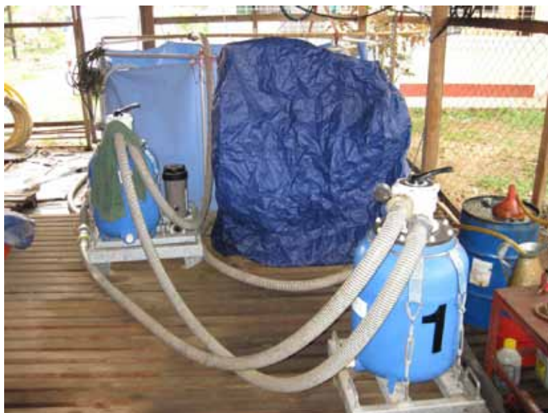
Water treatment unit deployed in Myanmar after Cyclone Nargis
