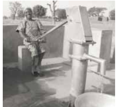
Woman using lengthened handle of water pump 97
