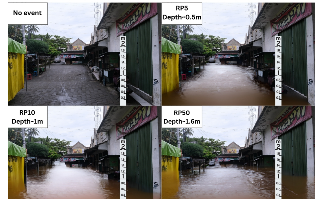
Figure 71. Photo of "Commercial Centre" area, a selected area of interest, with overlaid simulated flood levels for a 12hr storm for each event for return periods of 5-year to 50-year Source: F12-THK, 2024
