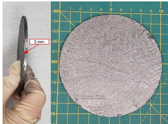
Figure 5.14 - \varnothing 100 mm D2-100 disk viewed from the side and from the face (FAST/SPS temperature: 950 °C, pressure: 50 MPa, dwell: 1 min)
