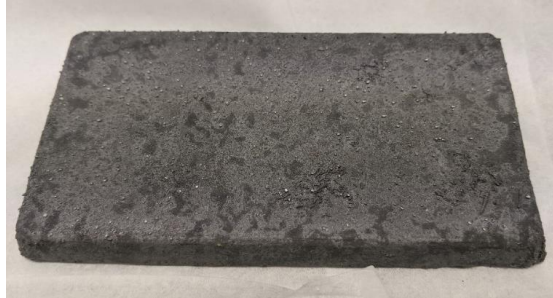
Fig. 5.1: Brick of pure \text{Cr}_2\text{AlC} obtained after solid-liquid state reaction (Image courtesy: Melina Poll).
