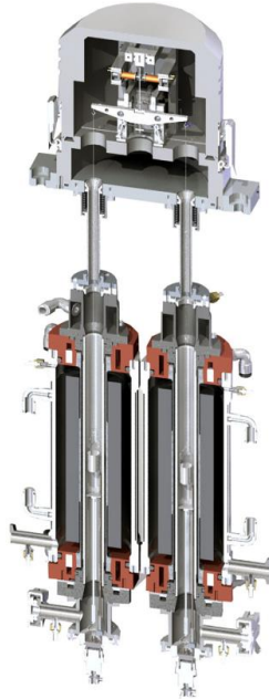
Fig. 4.2: Cross-sectional schematic of a symmetrical TGA setup, showing the microbalance on top with two identical furnace chambers below, one for the reference sample and one for the sample to be oxidized [164].
