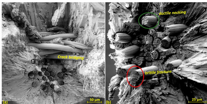
Figure 14. Representative fracture images of type 2 for both composites, images taken with SEM Carl Zeiss LEO DSM 982. (a) illustrates crack bridging, and (b) depicts ductile necking in the green-marked region and brittle fracture in the red-marked region.
