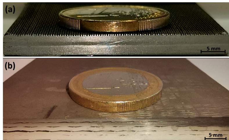
Figure 8. Solid composites of six layers via CVD: Fabric 1 (a), Fabric 2 (b).
