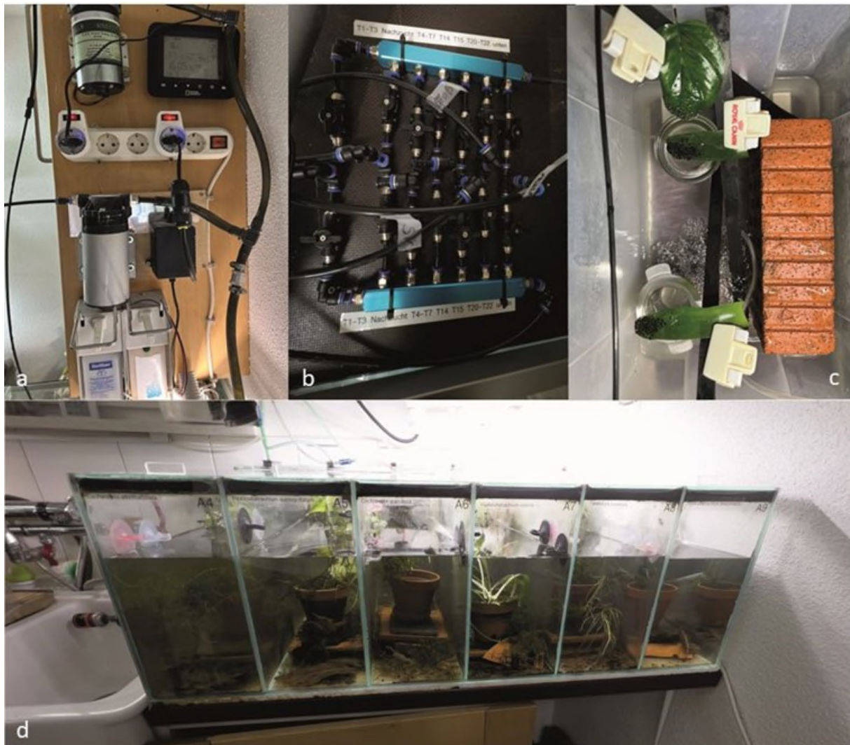
Fig. 39: Technical equipment for keeping and breeding glassfrogs (all photos by T. Eisenberg) a Measurement and control technology: switching relays as clock generators for pulsating irrigation systems b Switch panels for alternating use of different pumps of the irrigation system to enable pulsatile irrigation for individual terrarium groups c View into the humid chamber – the leaves with the eggs are attached above the water surface. A mist nozzle or an ultrasonic nebulizer regularly moistens the clutches with water. It is important that the leaf surfaces are allowed to dry for some time afterwards so that the eggs do not slip into the water prematurely. This clutch treatment is essential for the incubation of Cochranella granulosa clutches d Aquarium system for rearing glass frog tadpoles: one species is reared in each compartment. Note the airlift sponge filters for aeration and filtration of the water as well as numerous shelters for the larvae.
