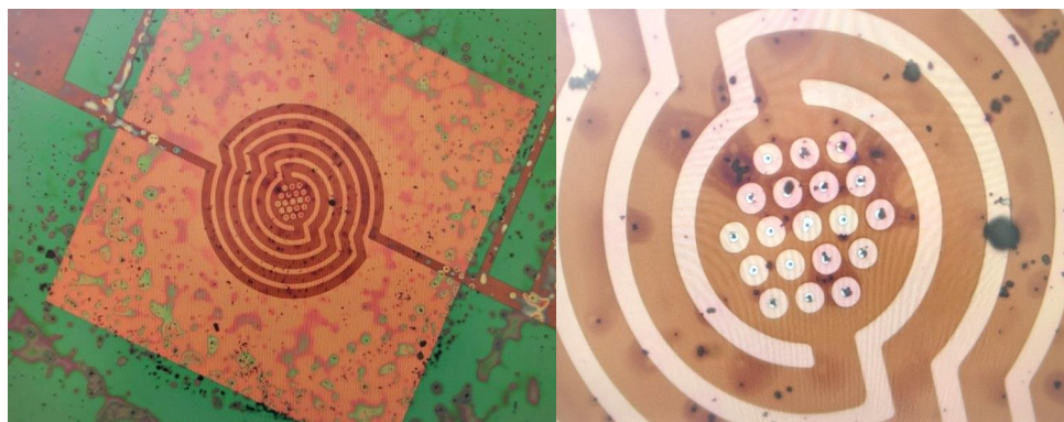
Figure 11.2: Optical microscopical image of MEMS heating chips. Left: SiN membranes centred in heating spiral (5x magnification). Right: SiN-windows loaded with Pd(NO 3 ) 2 supported on ZnO, which is visible as dark particles (50x magnification). Figure is taken with permission from reference 200 .
