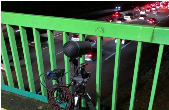
Fig. 2. Microphone set-up facing the A4, 93160 Noisy-le-Grand, France
