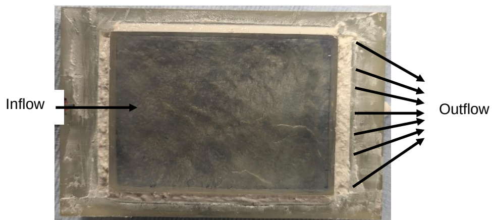
Fig. 3.70 3D printed test cell, including realistic fracture surfaces
