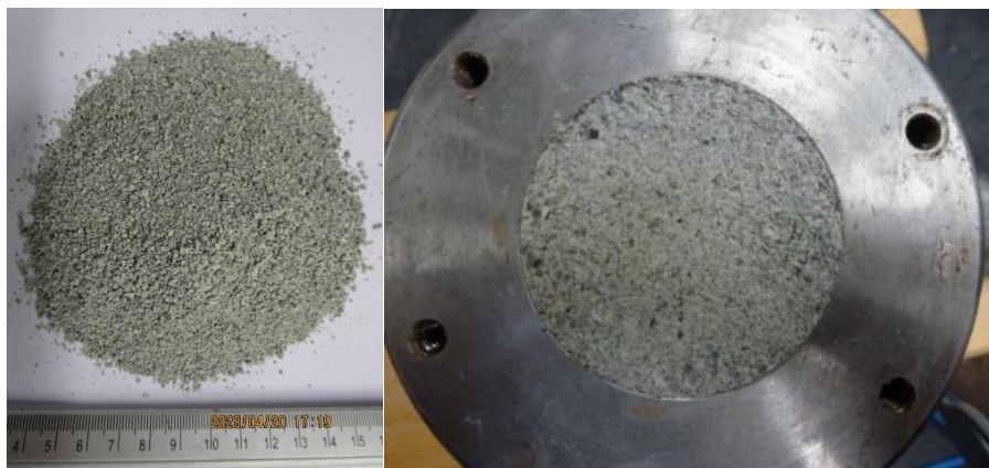
Fig. 3.31 MX-80 bentonite in the original granular form (left) and compacted in the test cell (right; from /KRÖ 19/)
