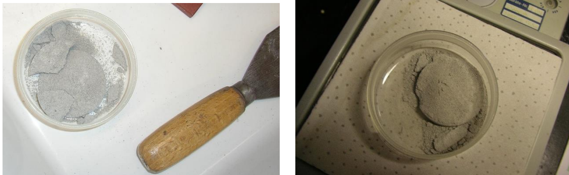
Fig. 3.34 Bentonite sample after scraping off (left) and weighing (right)
