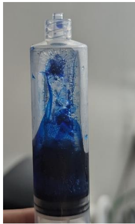
Fig. 3.71 Syringe filled with partially frozen 0,05% methylene blue solution; dark color: solution in liquid form; light blue: partially frozen; transparent: frozen
