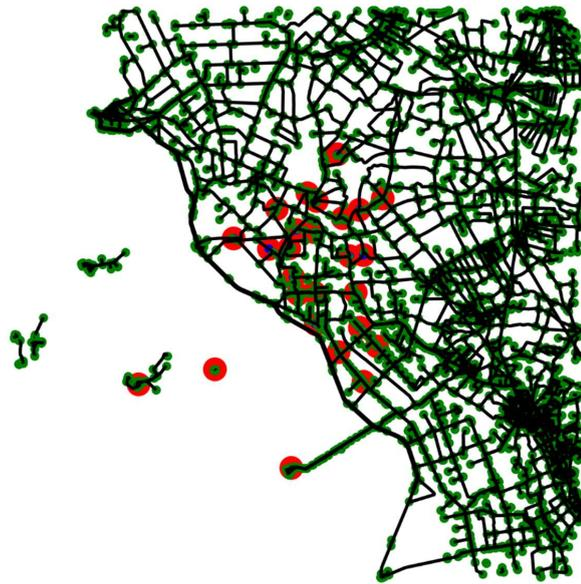
Figure 5-17 Road infrastructure in close proximity to the connection points, retrieved using Algorithm 3
