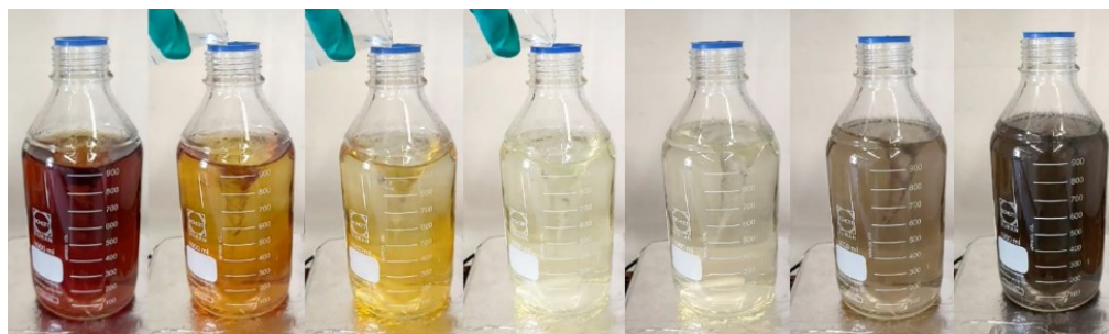
Figure 45. The color change of solution for 15 seconds from the moment that the reducing agent ( \text{NaBH}_4 ) was added.
