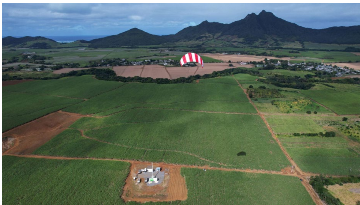
Figure 3 The SkySails Power airborne wind energy system in Mauritius (Courtesy of the SkySail Groups).
