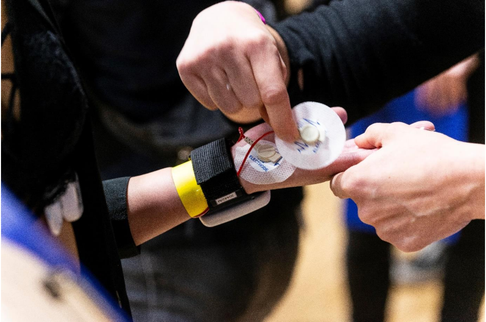
Figure 7: Attaching the EDA electrodes to the palm of a subject's non-dominant hand.
