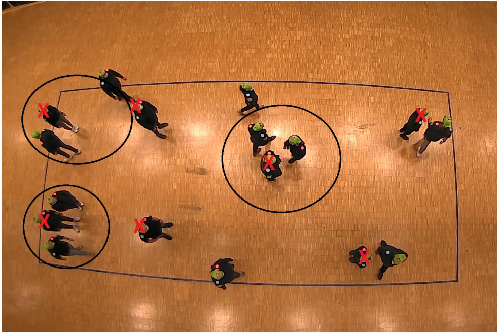
Figure 26: Camera snapshot of the short-term violation of personal space experiment. The red X marks the standing subjects. The black circles mark the problematic situations.
