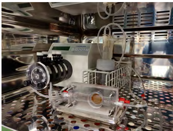
Figure 8: A live-imaging compatible flow chamber for testing biohybrid implant materials. A roller pump drives a closed fluid loop containing calcification medium, while the flow chamber exposes the sample within to physiological shear stresses like those seen in the vessel wall.
