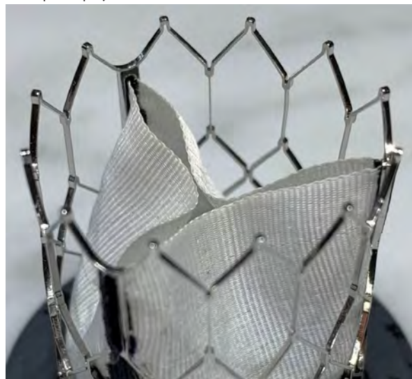
Fig. 1: Materials for Medical Devices: Textile heart valve tested with 200 million load cycles
