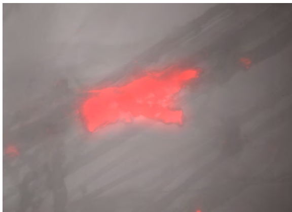
Figure 7: Calcified bovine pericardium after 7 days in calcification medium. Collagen fibers can be seen in the brightfield. A large, calcified lesion is seen in red, labelled with fluorescent Fetuin-A-mRuby
