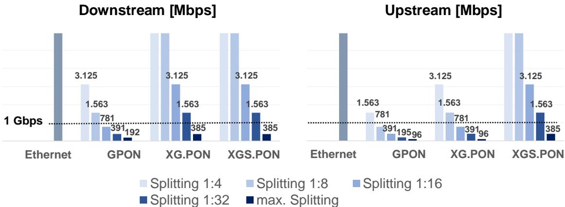
Source: WIK. The maximal splitting ratio is set at 1:1 for Ethernet PtP, 1:64 for GPON and at 1:128 for XG.PON and XGS.PON.
