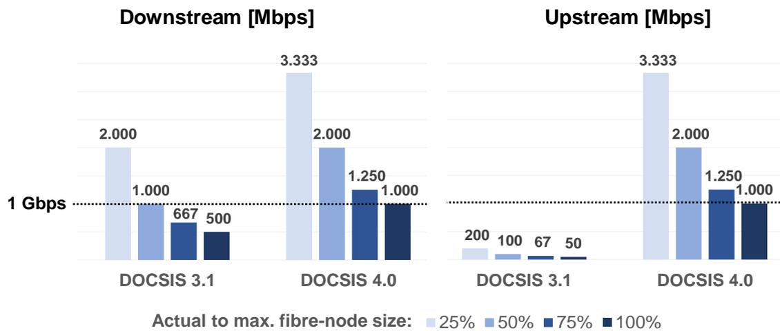
Source: WIK. The maximal capacity of a fibre-node is estimated at 100 connections for DOCSIS 3.1 and at 50 connections for DOCSIS 4.0.
