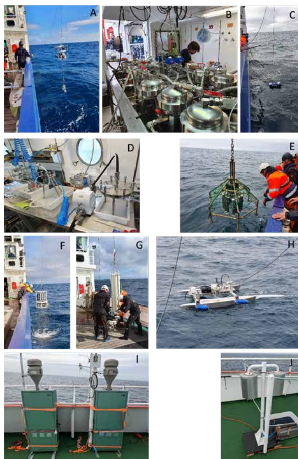
Figure 2: Sampling devices used on He578. A: in situ pumps; B: COMPASS filtration system; C: Sampling buoy with separate on ship pump/filtration set up (D); E: Multicorer; F: CTD; G: Marine Snow Catcher; H: Neuston catamaran with net and on board pump/filtration setup; I & J: High (I) and low volume (J) air sampler.
