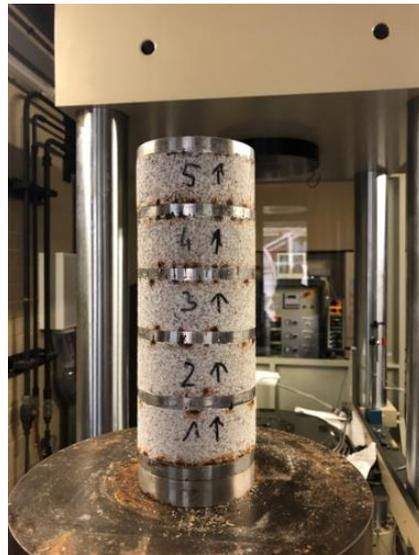
**Fig. 3.8** Pre-compaction experiment with distance pieces. Crushed salt was filled in five equal layers with defined material weights, lightly compacted to get a flat surface
