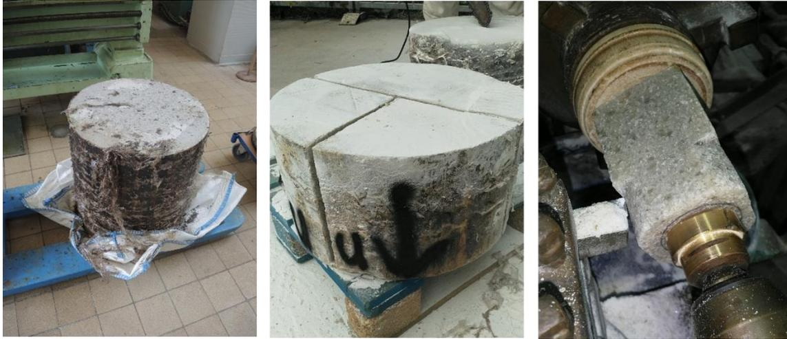
**Fig. 3.24** The compacted body was pressed out from the cell after finishing the test. From this large-scale sample several smaller sized cylindrical samples ( $l = 80\text{mm}$ ,  $d = 40\text{mm}$ ) were prepared by sawing small segments and machining with a lathe
