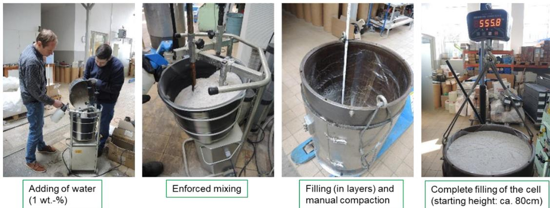
**Fig. 3.14** Preparation of the „large IfG oedometer cell“: Salzgrus (initial state as delivered, pre-treatment (homogenization) and stepwise filling and weight control of the cell
