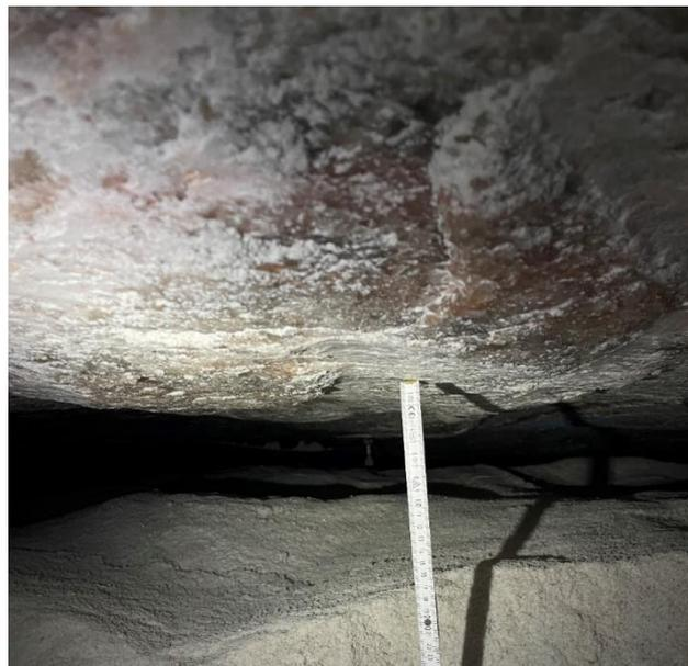
**Fig. 2.15** Measurement of gap between the KOMPASS backfill body and the roof of the drift /SCH 23/
