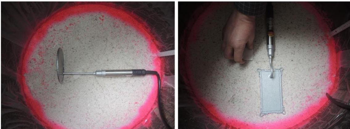
**Fig. 3.26** Two hydraulic pressure cushions were installed in the lower third of the filled cell while filling it with the crushed salt material. One records the horizontal, the other records the vertical acting pressure
