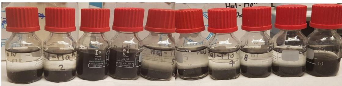
**Fig. 8.2** Experimental batches of molybdenum(IV) in halite/ anhydrite-saturated solution
