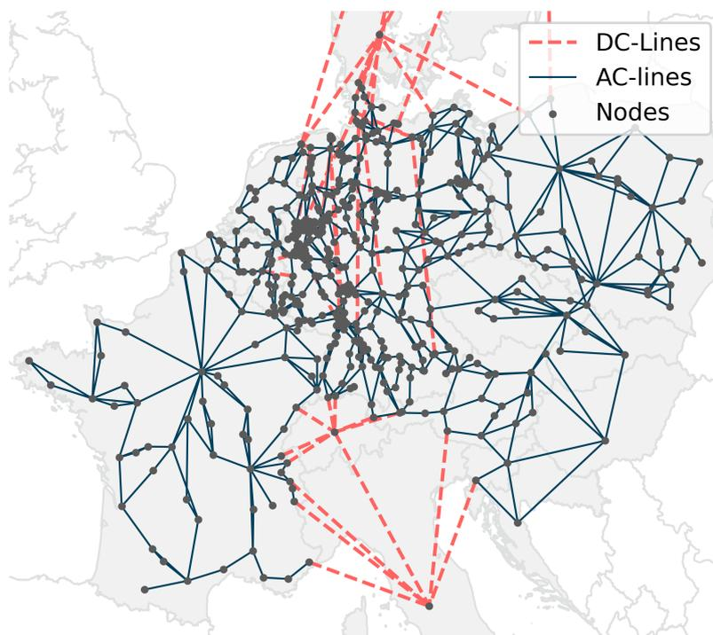
Figure 1: Modeled transmission grid after grid reduction
