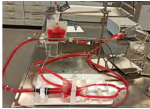
Fig. 8: Test setup with ghost blood and left atrium appendix model.
