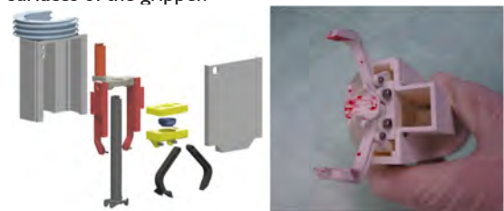
Fig. 6: Gripper designed for toolless disassembly (left), test contamination with sheep blood (right)
