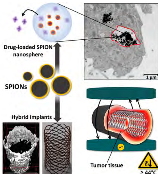
Fig. 6: Sketch of SPIONs consisting of a metallic core with a stabilizing organic shell. They can interact with the cell directly delivering drugs to the cell. Further, SPIONs inside hybrid implants can be activated in an alternating magnetic field to generate local heat and destroy neighbouring cancer tissue (DOI: https://doi.org/10.3390/nano11030618 ).
