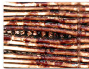
Fig. 13: Microscopic view on in vitro cultivated thrombus in ECMO oxygenator.
