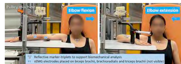
Fig. 18: Experimental setup. The subject's arm is connected via a sling to a pulley machine. The horizontal armrest provides stability and standardizes the movements performed.
