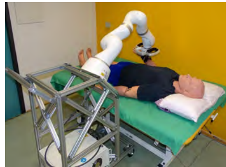
Fig. 25: PflerKoRo prototype. Its robotic arm holds the arm of a simulated patient.
