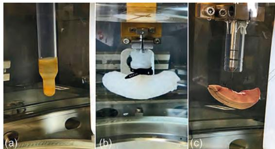
Fig. 1: Different in-vitro setups: latex holder (a), kidney phantom (b) and porcine kidney (c).
