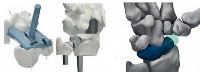
Fig. 5: A patient-specific instrumentation and wrist implant (left) and a patient-specific spacer (right)
