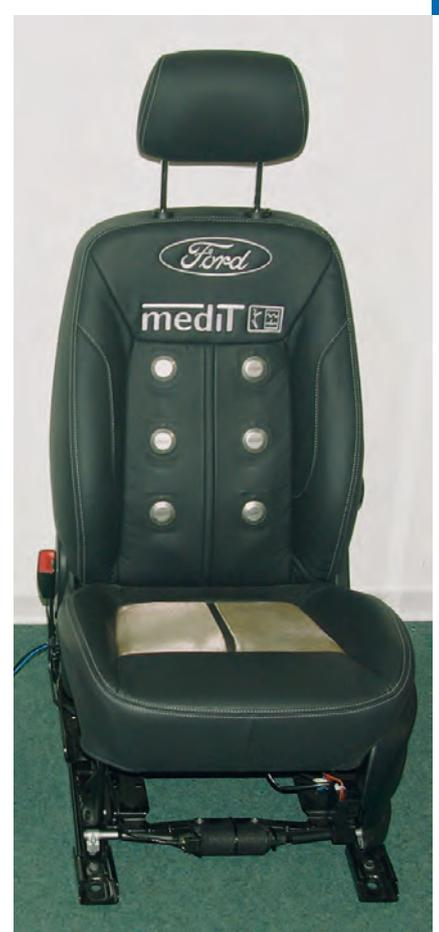
**Fig. 9:** Multi-channel cECGs integrated in a car seat.
