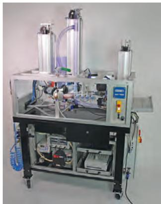
Fig. 15: Fully automated mock circulation loop for in-vitro tests of the ReinHeart TAH physiological control.
