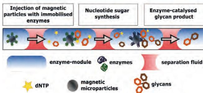
Fig. 1: Automated enzymatic glycan synthesis in a compartmented flow microreactor system.
