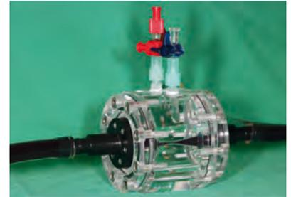
Fig. 11: Non-haemolytic flow loop resistance.
