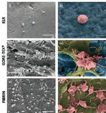
Fig. 4: Assessment of hemocompatibility by evaluation of adhered platelets based on SEM images. While elastin-like recombinamers (ELR) surfaces presented minimal platelet adhesion, activated (pink) and fully activated platelets (golden) were covering GoreTex and fibrin surfaces. Substrate surfaces are coloured in blue.
