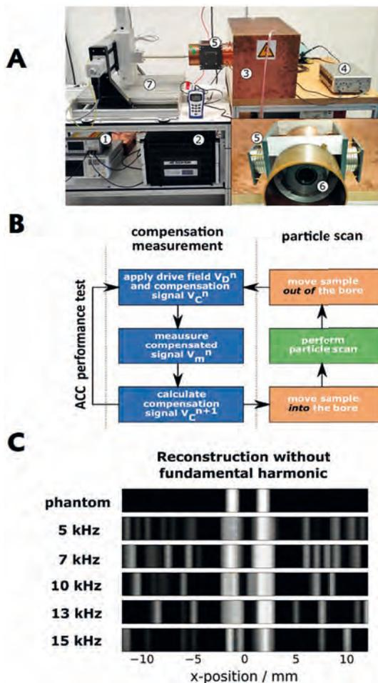
Fig. 2. A: Experimental setup for multifrequency magnetic particle imaging (mf-MPI): B: Flow chart of the active compensation control. C: Comparison of phantom image reconstruction with and without fundamental harmonic information. The applied drive field frequencies were 5, 7, 10, 13, and 15 kHz.
