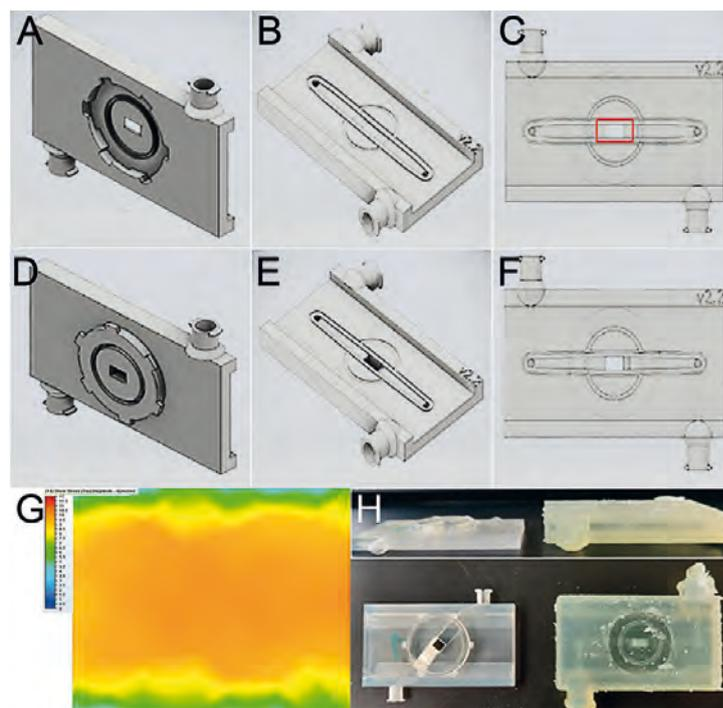
**Fig. 4: 3D-printed microfluidic device for vessel-on-a-chip culture.**
