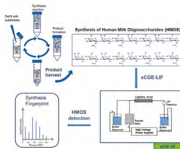
Fig. 2: Combination of repetitive batch-mode synthesis of nucleotide sugars with HMOS synthesis to create an analytical HMOS fingerprint database.
