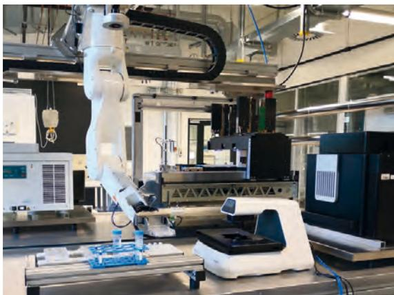
Fig. 4: iPS cell production and differentiation in automatic cell production facility (iCellFactory).
