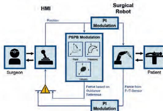
Fig. 7: Principle of Cooperative Bilateral Telemanipulation
