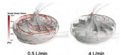
Fig. 14: Shear stress simulation in the 'Revolution 4' pump at low (left) and high (right) flow.
