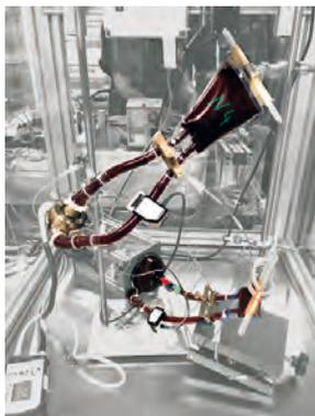
Fig. 10: Small-volume test loops for blood pump testing.
