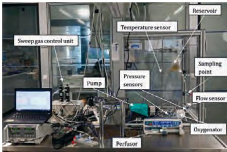
Fig. 9: Test bench for long-term oxygenator testing.
