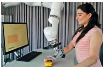
Fig. 19: Performance of a rehabilitation exercise using robotic guidance and assistance. Feedback about and real-time monitoring of movement paths is provided via the system's integrated display screen.
