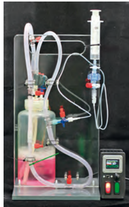
Fig. 4: The VascuTrainer bioreactor system with a medium reservoir, a centrifugal pump, pressure and flow sensors, a pump control unit and the tissue-engineered vascular graft (TEVG).
