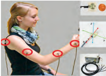
Fig. 18: Assessment and evaluation of movement quality e.g. in upper extremity using inertial sensors
