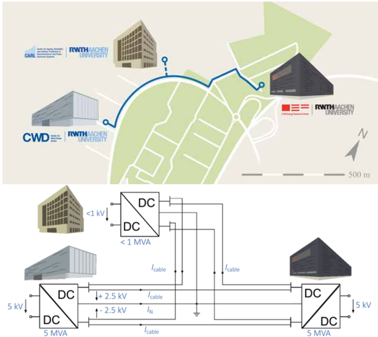
Figure 8.6 The RWTH 5 kV MVDC Campus grid connects the 4 MW Center for Wind Power Drives (CWD) with the 5 MW test hall of E.ON ERC|PGS. The bottom picture shows an elementary schematic. A low-voltage connection to the Center for Aging, Reliability and lifetime Prediction of Electrochemical and Power Electronic Systems (CARL), which has a 100 kW photovoltaic system and large battery test infrastructure, is planned. The MVDC can exchange energy between the centers, avoiding peak loads and decreasing the cost of operating them [14].
