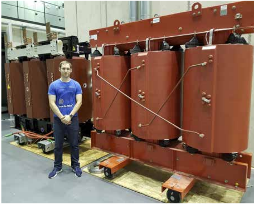
Figure 8.4 Dr. P. Joebges standing next to a 4,5 MVA, 50 Hz dry-type distribution transformer. With a total weight of 11.5 tons, 2.5 kg per kVA is needed (with permission).
