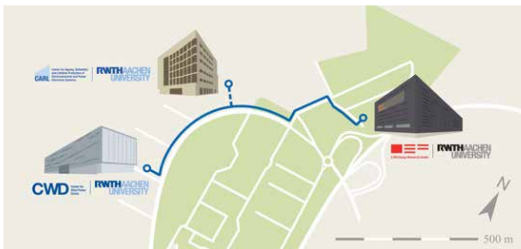
Figure 1.8 The bipolar 5 kV campus grid is installed at RWTH CAMPUS Melaten and creates a MVDC connection between the substations of two laboratories (PGS and CWD). The Center for Aging, Reliability and Lifetime Prediction of Electrochemical and Power Electronic System is scheduled to be connected to the MVDC Grid.
