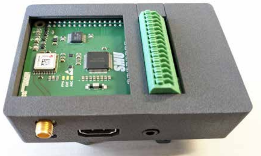
Figure 1.5 The synchronized measurement unit (SMU) and automation blockchain technology, developed by Prof. Ponci, offers a low cost end-to-end monitoring and data exchange solution for energy communities.
