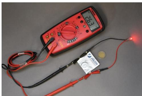
**Figure 51** Photograph of the pressure-free Na/NYS/S pouch cell and the powered light-emitting diode.
