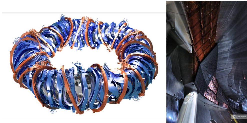
Figure 2.5. Left: schematic view of the Wendelstein 7-X stellarator with its twisting geometry and magnetic coils surrounding the vacuum vessel [11]. Right: View inside the Wendelstein 7-X stellarator [8].
