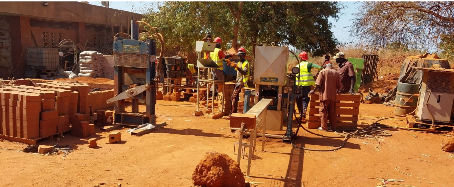
The production process of compressed earth bricks, Senegal. © GIZ Senegal/Fatou Ndoeye
