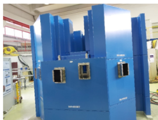
Figure A.9: iii) Assembly of the stationary part of the shielding
