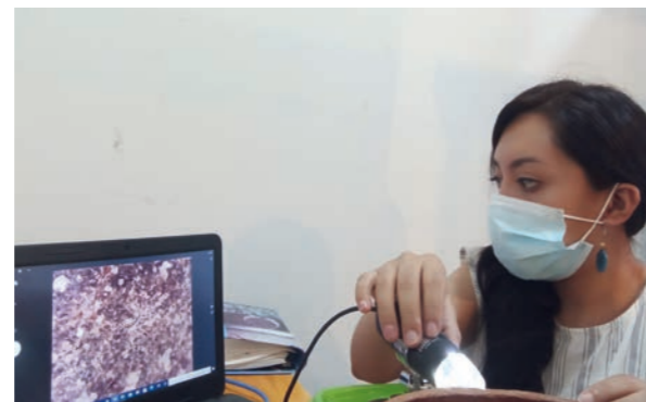
Pottery analysis with a portable microscope.
