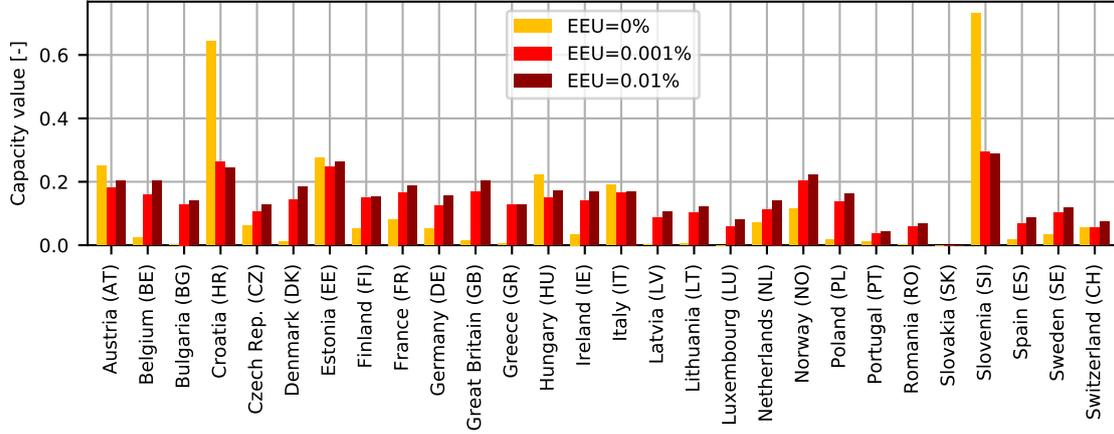
Figure 9: Region-specific capacity value of wind power with respect to total system (EU) for different reliability levels EEU
