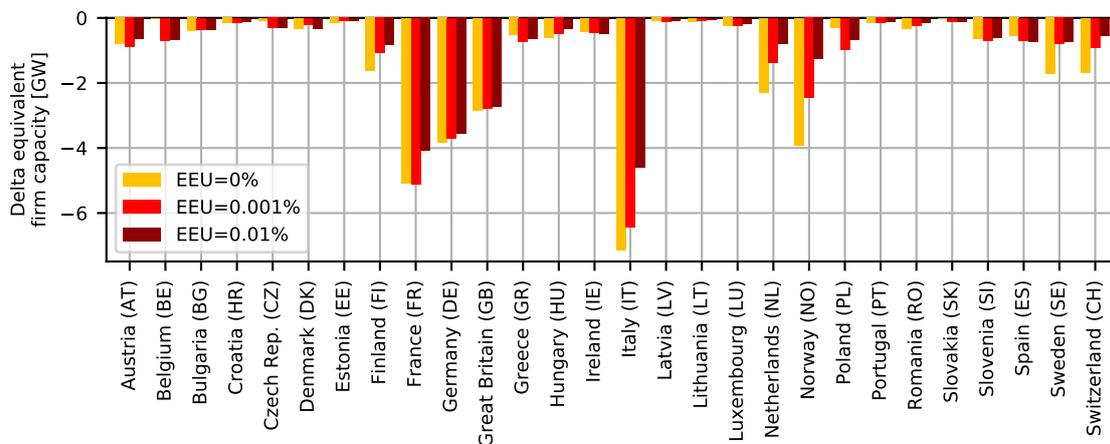
Figure 6: Gains from cooperation: Reduction in equivalent firm capacity with cooperation of total system (EU), compared to isolated regions
