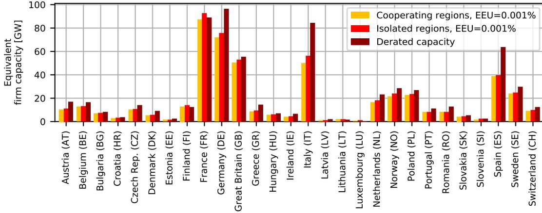
Figure 7: Equivalent firm capacity for isolated and cooperating regions compared to existing derated capacities
