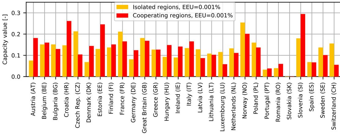
Figure 8: Region-specific capacity value of wind power with respect to total system (EU) for isolated and cooperating regions
