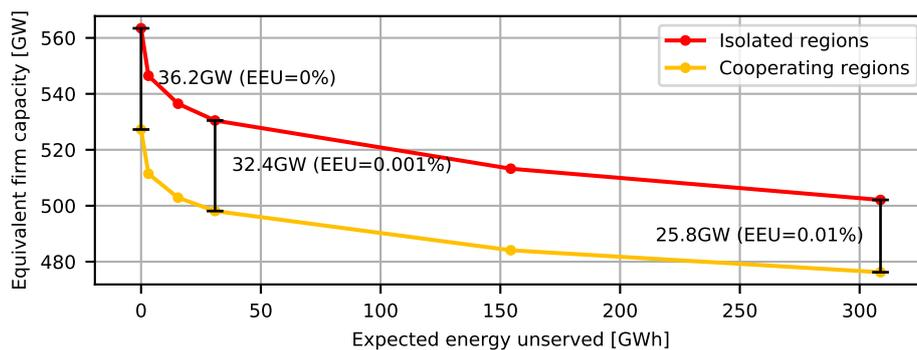
Figure 5: Capacity requirements aggregated over Europe as a function of EEU with the respective gains from cooperation (marked in black)
