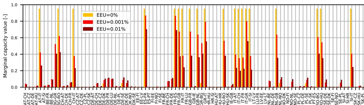
Figure 12: Marginal capacity values of interconnectors between two regions with respect to total system (EU)
