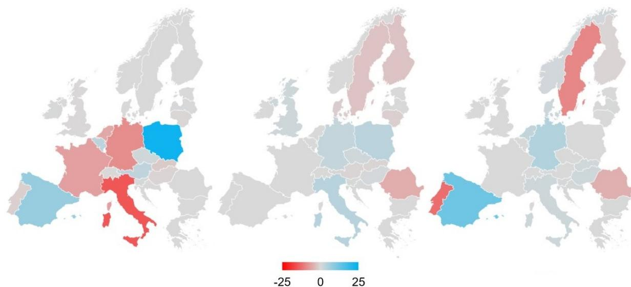
Figure 5: Net imports and exports of gas mix (left), ptx liquefied hydrogen (middle) and ptx diesel (right) in  $\text{TWh}_{\text{th}}$ , with positive values in blue indicating net import and negative values in red indicating net export
