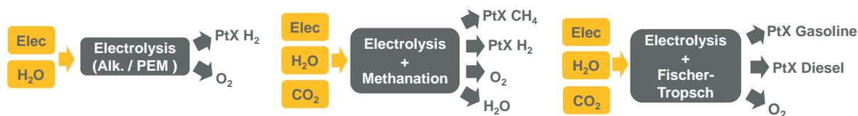
Figure 2: Inputs and outputs of ptx processes
