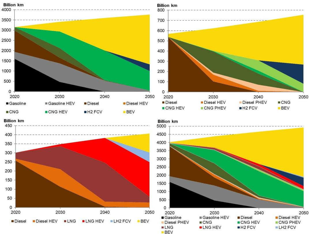
Figure 3: EU vehicle mix up to 2050 for PPVs (top left), LDVs (top right), HDVs (bottom left) and all vehicles (bottom right)
