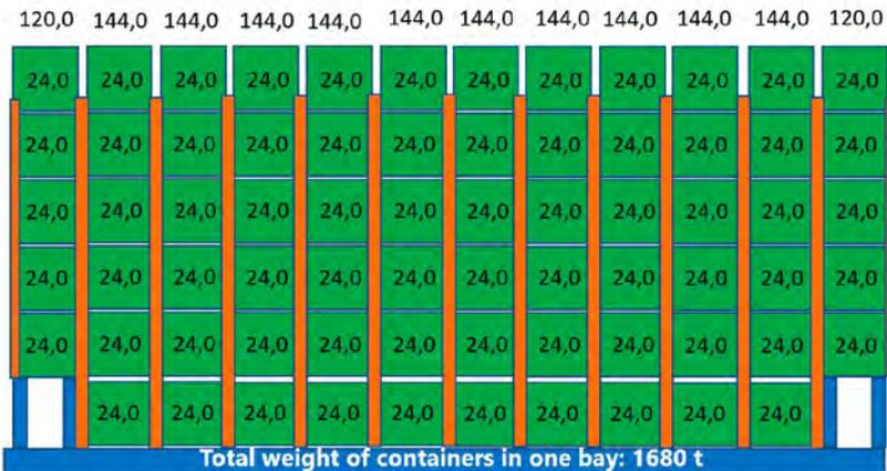
Abb. 19: STACK WEIGHT DISTRIBUTION WITH CELL GUIDES
