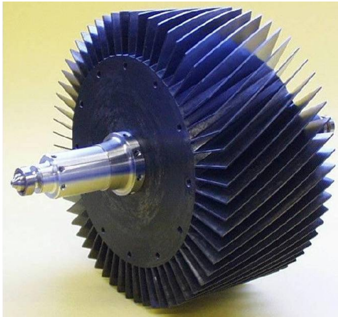
Fig. 15.6: Photo of the velocity selector drum of the JCNS instrument KWS-3 showing the screw-like twisted channels separated by absorbing walls, which only neutrons of a certain wavelength band can pass when the drum is turning.
