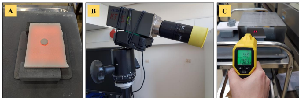
Figure 2. 10: Furnace thermal cycling setup: (A) porous \text{Al}_2\text{O}_3 plate with sample taken out of the furnace, (B) high-temperature pyrometer, (C) low-temperature laser pyrometer.
