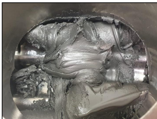
Figure 4. 2: Consistency of a monolithic 50 vol.% \text{Ti}_2\text{AlC} feedstock upon mixing in a duplex kneader at 170 °C.
