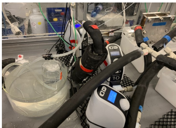
Figure 5.23 Setup for the test of Faradaic efficiency by water displacement.
