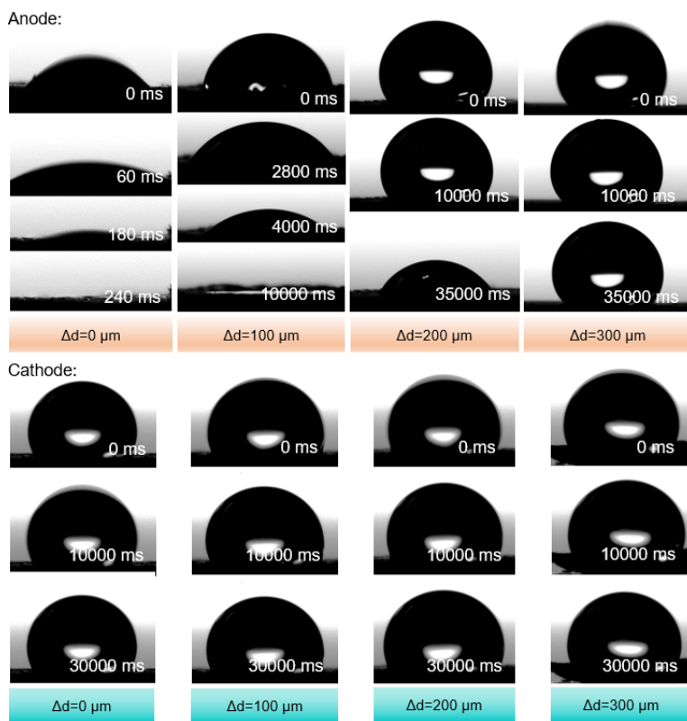
Figure 7.5 Water contact angle of anodes with Ir coated on the Ni fiber and cathodes with Pt/C coated on the carbon fiber, captured at different time.
