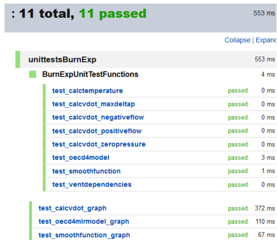
Figure 4 Example of a test report for the unit testing, in which the separate functions are tested before being used in the simulation
