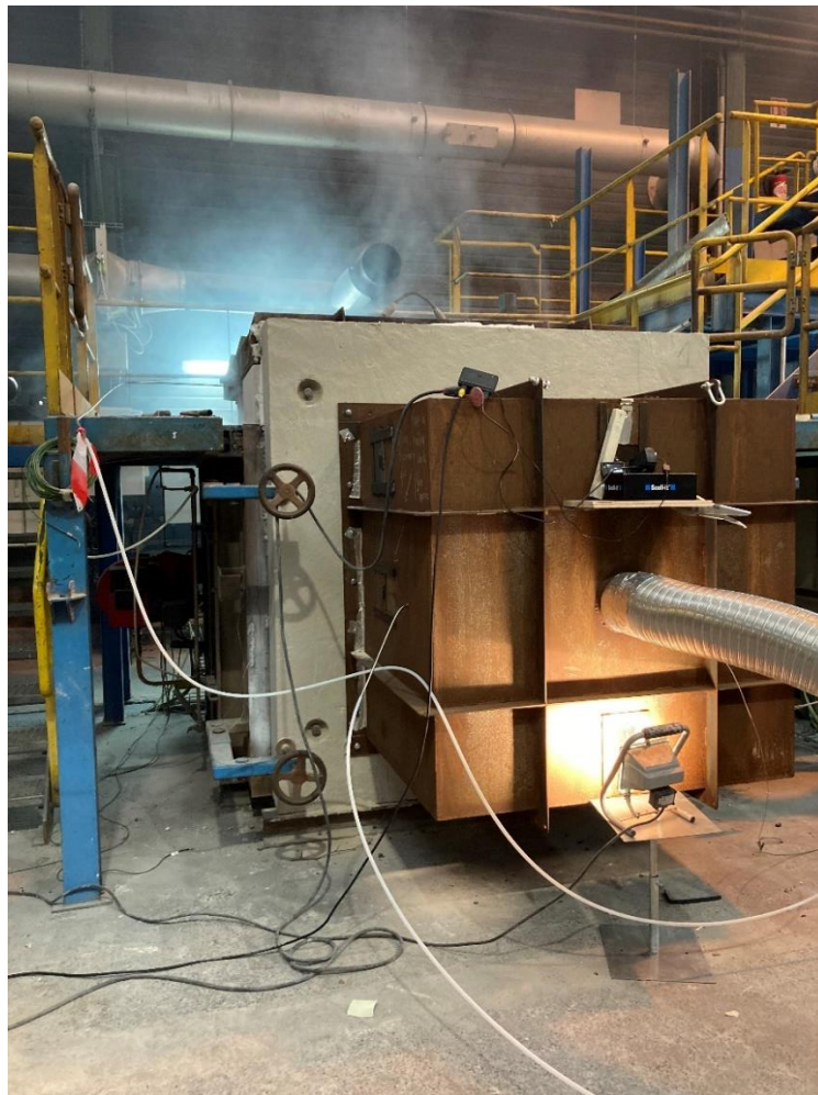
Figure 5 Pressure vessel implemented on the test mock-up in the wall
