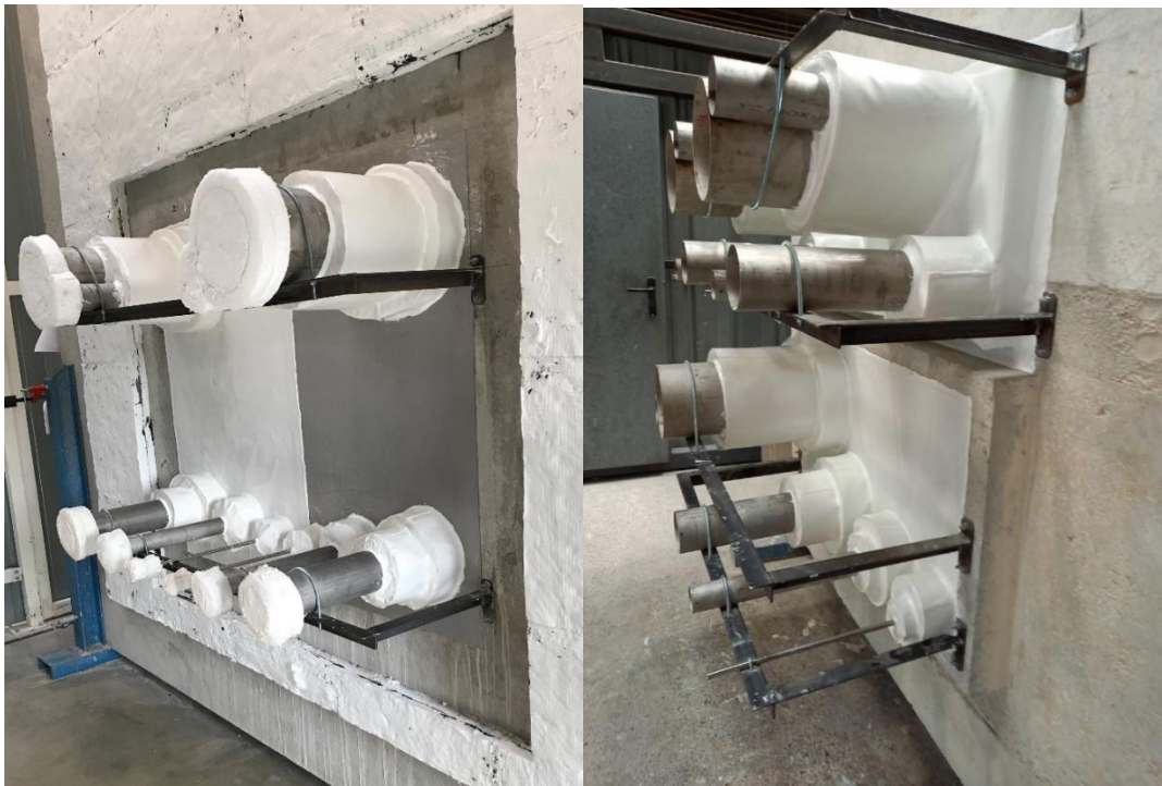
Figure 7 Example of the mock-up for the fire tests of penetration seals
