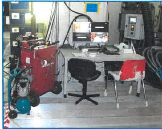
Figure 2 Monitoring station with control panel and monitor outside the hazardous zone
