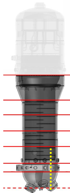
Figure 1 Wire saw cuts through the steam generator
