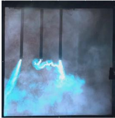
Figure 4 Open box experiment OB2 (copper electrode, 1000 V, 15 kA)
