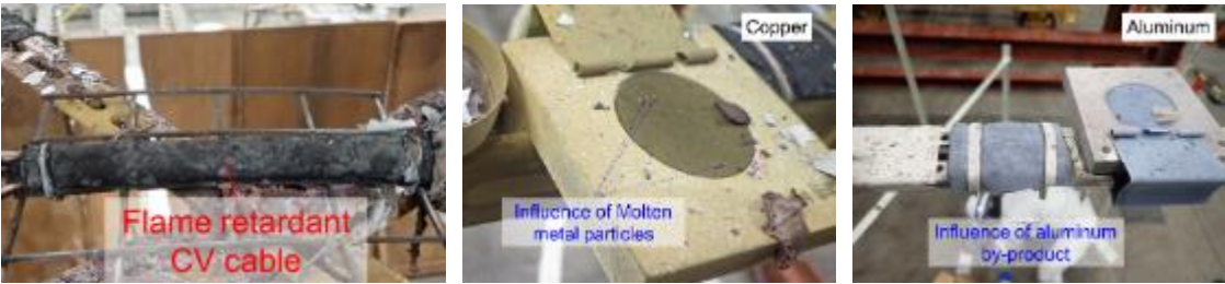
carbonization of the cable jacket (left), influence of copper and aluminum by-products
