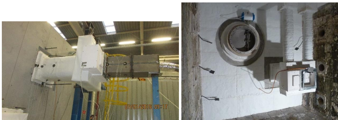
Figure 6 Picture of damper tested; 300 mm x 300 mm (left), and 600 mm section and 300 mm x 300 mm (right)
