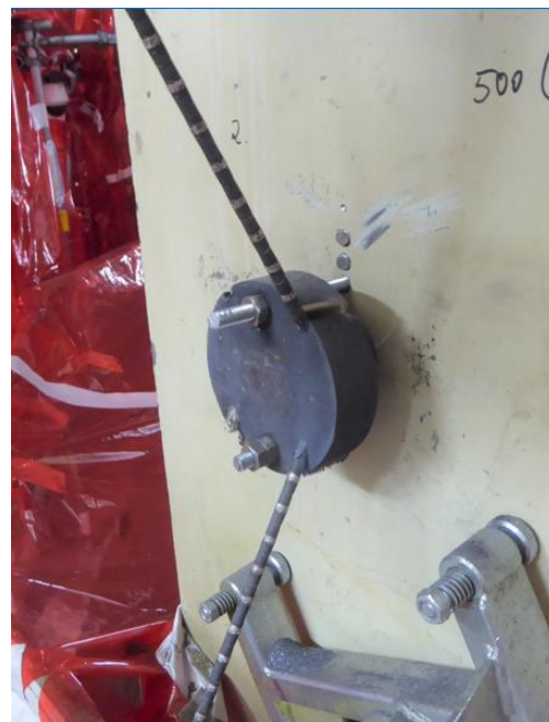
Figure 9 Test setup (top) and on a spacer 50 % cut with new wire (bottom left) and 90 % cut with depleted wire (bottom right)
