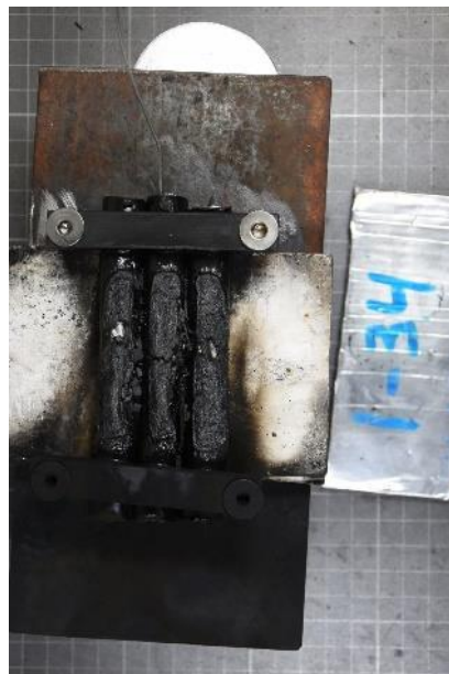
Figure 7 Solar Furnace Test 1-34 (3 cable bundle, \sim 25 \text{ MJ/m}^2 )
