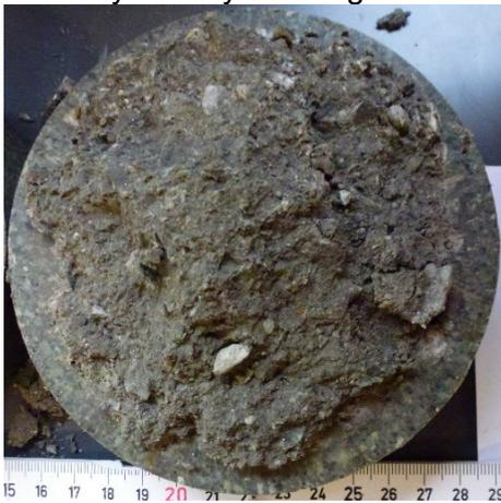
Seal 3: claystone/bentonite (7/3)-blocks with bentonite-filled gap and joints
