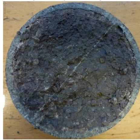
Seal 4: claystone-blocks with bentonite-filled gap and joints
