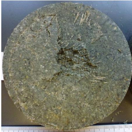
Seal 1: compacted bentonite pellets/powder mixture
