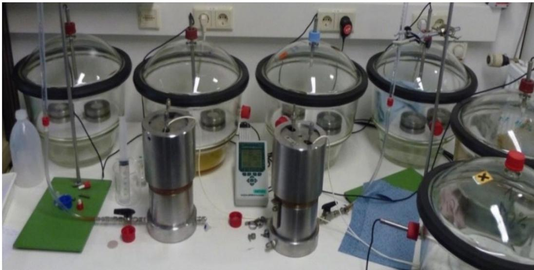
b. Samples placed in desiccators at different relative humidities
