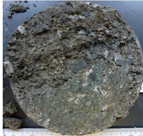
Seal 2: compacted claystone/bentonite (7/3) mixture
