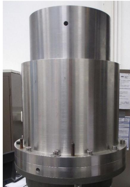
**Fig. 2.12** A large oedometer setup for compaction of barrier materials
