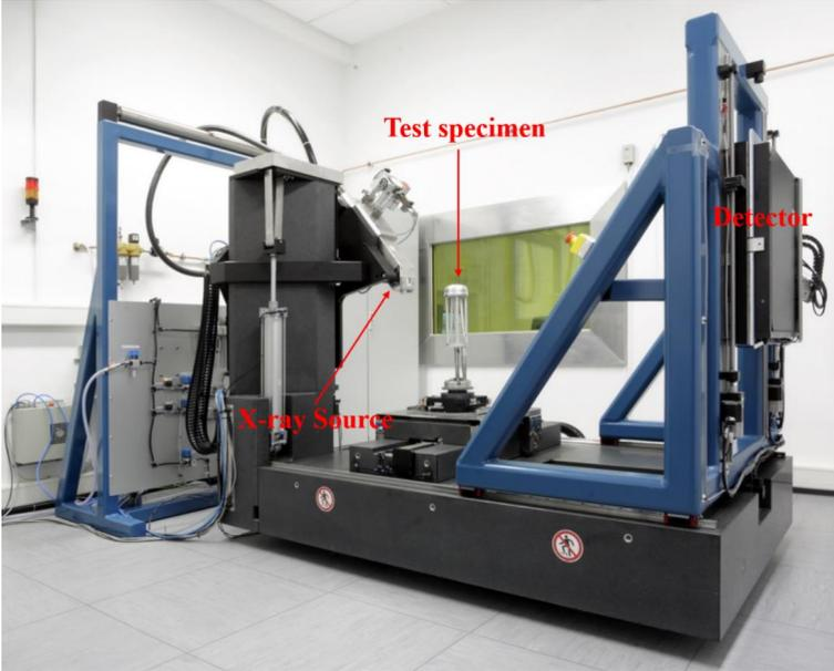
Fig. 3-7. Open X-ray computed tomography system at ZEA-1
