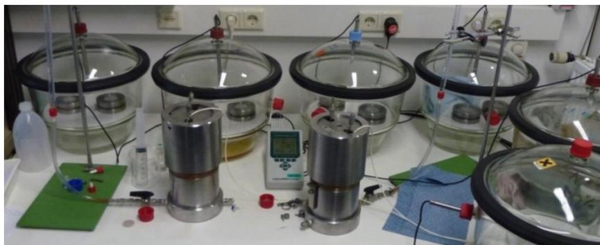
b. specimens placed in desiccators at different relative humidities
