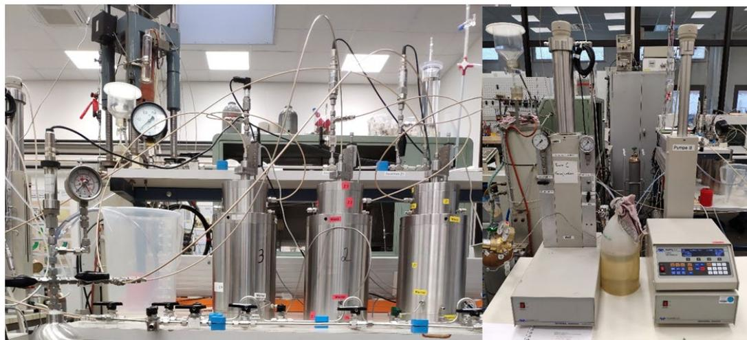
**Fig. 2.21** Setup of the gas penetration testing on three parallel specimens in coupled triaxial cells
