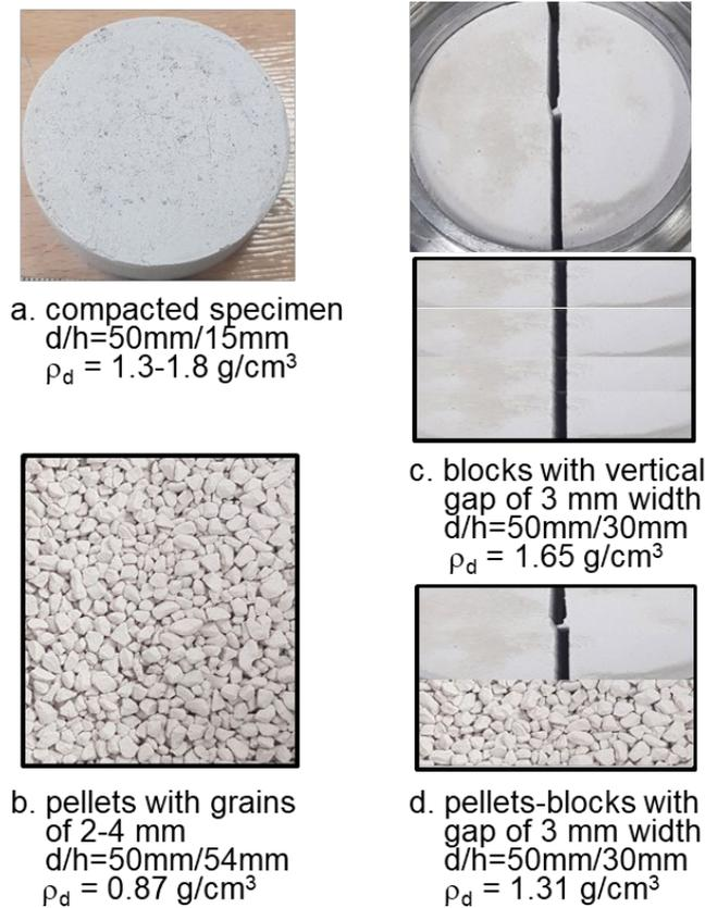
**Fig. 2.8** Different kinds of specimens prepared using GMZ01 bentonite
