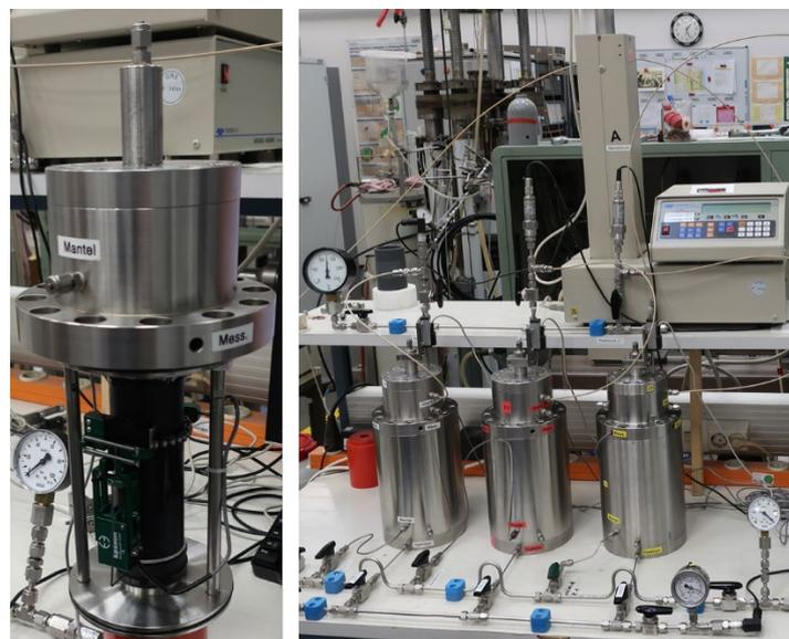
**Fig. 2.29** Setup of the gas penetration testing under constant volume
