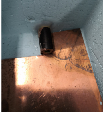
Figure 3.12: Picture of the copper plate mounted to the cold-finger of the CFH-CO 2 . with a minimum temperature of -116.18^{\circ}\text{C} , 17.88^{\circ}\text{C} less than inside the chamber. In order to improve the efficiency of the cooling agent, a copper plate was mounted at the CFH cold finger as shown in Fig. 3.12. Copper has a high heat conductivity of 386\text{ W m}^{-1}\text{ K}^{-1} at standard conditions which increases with decreasing temperatures (Carvil, 1993). The temperature heat conductivity dependence of copper is shown in Appendix B in Fig. B.1. Within the temperature range relevant for atmospheric balloon profiles, the thermal conductivity of copper slightly increases to 413\text{ W m}^{-1}\text{ K}^{-1} at -73^{\circ}\text{C} . By enlarging the contact area of the cold finger to the cooling agent with the copper plate, the cooling efficiency is expected to increase. With this modified CFH a second test flight was performed. The results can be seen in the Fig. 3.13 and Fig. 3.14. As expected, the performance of this test flight shows improved cooling efficiency of the CFH-CO 2 . The temperature of both
