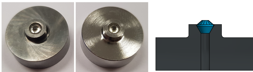
Figure 6.14: Bottom pistons made from Ni-WC ( left ) and NiCrAl ( center ) with mounted diamond, and schematic view of the bottom piston ( right ).
