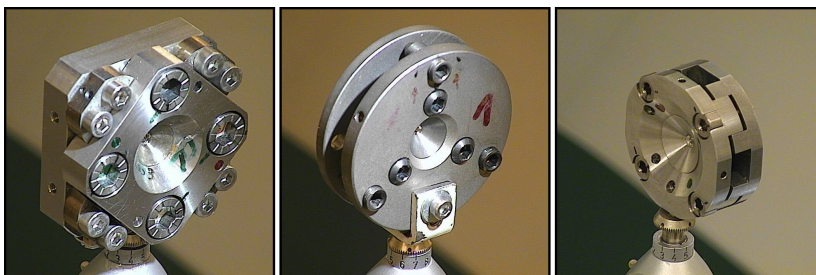
Figure 4.2: The three types of DAC used for experiments in the present work: (from left to right) Ahsbahs, Boehler-Almax and YaoDAC.
