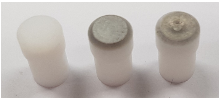
Figure 6.29: The PTFE plugs of the sample containers used for the clamp cells. Left : the regular PTFE plugs; ( center ): the PTFE plugs with the Al-layer on the top face; right : the PTFE plugs with the Al-layer after usage.
