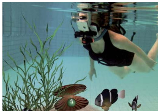
Underwater treasure quest: As a demonstrator Fraunhofer FIT created the world's first mobile underwater AR game. Its main component is a waterproof display in front of a diver's mask. The display lets the diver see his or her real underwater environment plus additional virtual objects.
