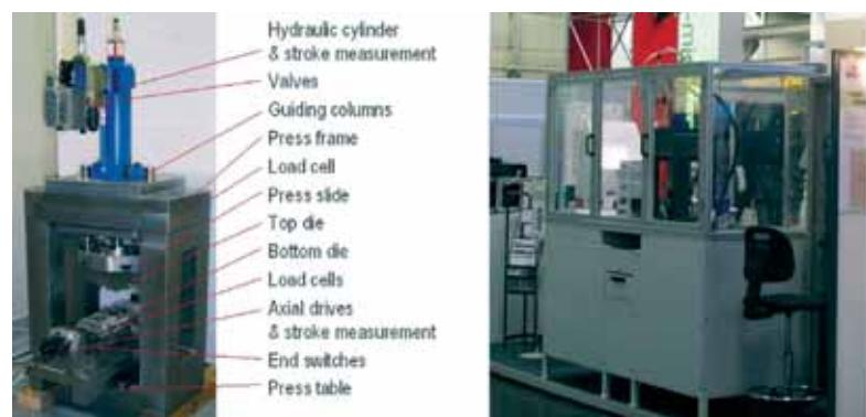
Figure 5: Micro-hydroforming prototype machine (hydroforming press and complete machine system)
