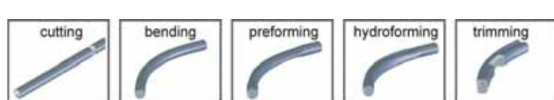
Figure 2: Typical process chain for hydroforming part manufacture
