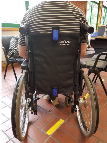
Figure 2.4: Participant sitting in a wheelchair that is equipped with IMUs.
