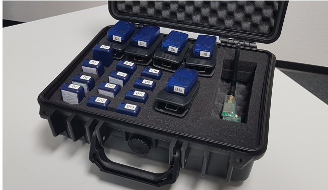
Figure 2.2: IMU sensors and hub device with an antenna.
