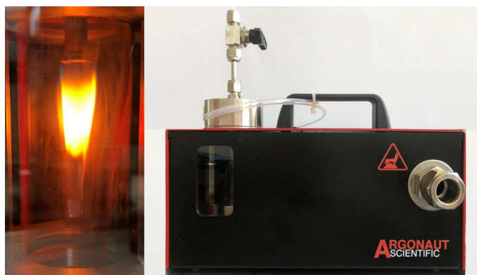
Fig. 32: The Miniature Inverted Soot Generator (on the right), and the image of an open-tip propane flame from the experiments on the left.
