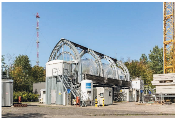
Figure 2. 1: Picture of the SAPHIR chamber. At the right side, the tower is seen at which the inlet line for ambient air was mounted in the JULIAC campaign. Copyright to: “Forschungszentrum Jülich / Sascha Kreklau“
